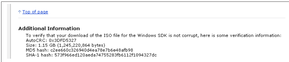
Figure 20-1. File hashes as a verification mechanism
