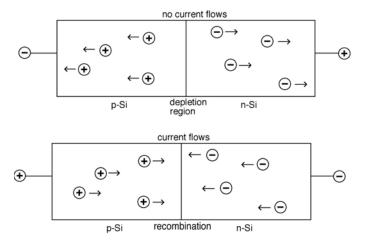
In order to travel from a valence band to a higher-energetic conduction band, electrons require an amount of energy equal to the energy differential, or band gap<sup>10</sup>, between both orbitals. This energy can be added via electric charge or heat. A semiconductor's material determines the band gap, as well as many other factors such as charge drift velocity that influence semiconductor performance.
