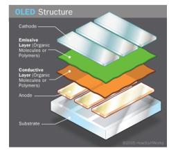
Basic OLEDs utilize two different types of organic materials, each suited for either HTL or ETL purposes and doped accordingly. One of these materials needs to be transparent so light can escape. OLED structures are aggregated as large grids, with each structure corresponding to a single dot or pixel. Emitted RGB photons need to be balanced to create white light. A substrate, which can be flexible or rigid, functions as a protective outer layer.
