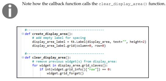
The clear\_display\_area() function knows both the row and column in which the widgets of tabs are being created, and by finding row zero, we can then use grid\_forget() to clear the display.
