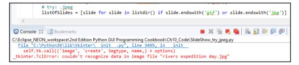
Using Pillow, we can display both .gif and .jpg files. After a successful installation of the Pillow package, we only have to make a few changes:
