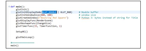
We create the TimerFunction() to be passed into glutTimerFunc(). In this function, we do some math to position the red square and make it bounce of the window walls. At the end of the function, we recursively call this function in glutTimerFunc():
